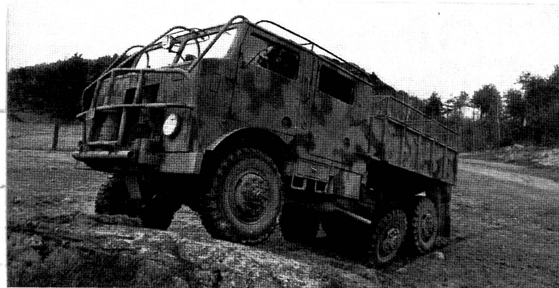
The TVC 6-wheel-driven artillery tractor.
